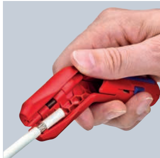
Stripping of a coax cable
