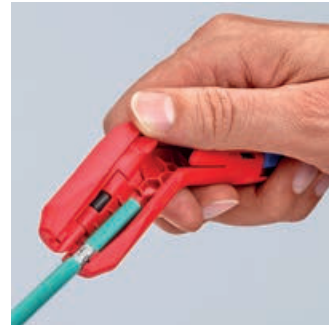
Stripping of a data cable
