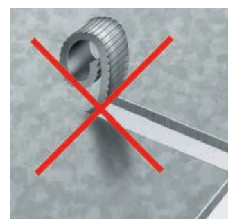
Notching without chip breaking
