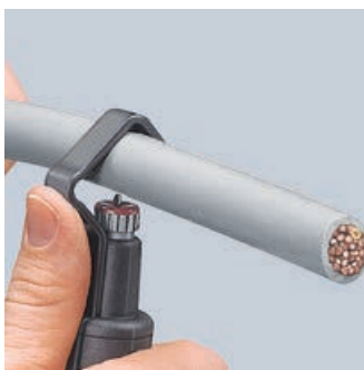
Setting the tool for circular cut
