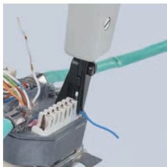
Inserts and cuts cables in one operation
