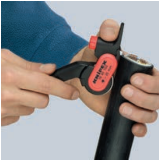
Setting the tool for longitudinal cut
